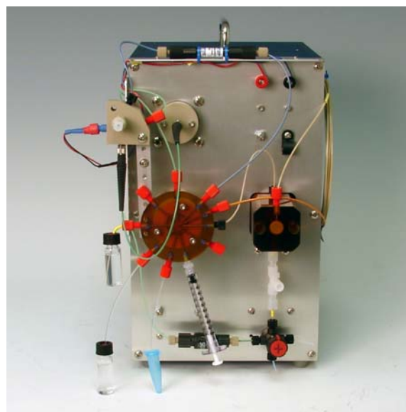
SICrom System configured with built in PMT Detector
