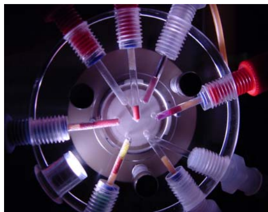
Example Custom System - Recycling Immunoaffinity Chromatography Unit with Built in Laser Induced Fluorometer
