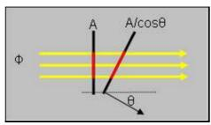
The correct measurement of spectral irradiance should include light from the entire hemisphere above the measurement plane.
