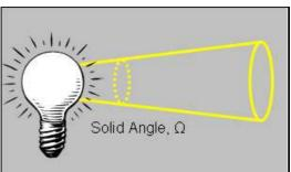
In its strict definition, radiance is measured using an input optic that measures over a defined area of the source, into a defined solid angle. It follows that the measurement instrument view is smaller than, or is overfilled by the source.
