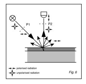
The light source emits unpolarized radiation, which becomes polarized in the 0°-plane by the filter P1. By passing twice through the ink layer the *ink modulated light* loses its polarity. Only the 90°-plane portion can pass the filter P2 and enter the photodetector. The reflected surface light stays polarized in the 0°-plane, and is stopped by P2. The photodetector thus measures just the light which passed twice through the ink layer, and so the value is not distorted by surface light.
