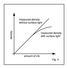
The influence of surface light is greater with matt surfaces than with glossy surfaces. Matt surfaces reflect a significant amount of light into the direction of the photodetector, whereas high gloss surfaces reflect most of the radiation directly without reaching the photodetector.
