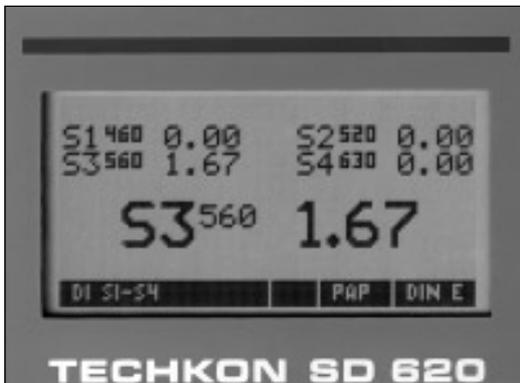
Optional choice of four additional filters for measurement of special colors (with automatic color recognition)
