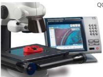
QC-300 features an array of video measurement tools, including simple crosshair measurement, manual or automatic single point detection and multi-point video edge detection.
