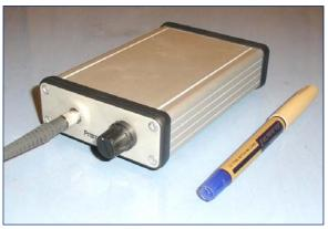
panel potentiometer. The Slim-LED is ideal for use with various fiber optic spectrometers in continuous measurement mode.
