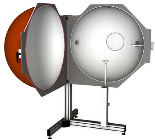
BTS2048-VL with a 1m diameter integrating sphere
