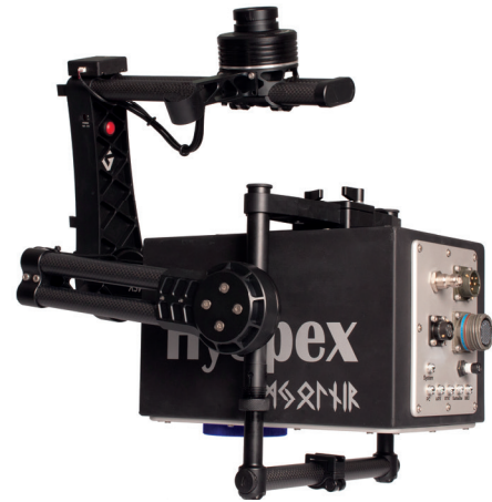
HySpex Mjolnir and Gremsy gStabi H16.
