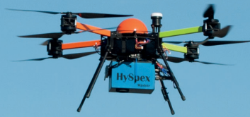
HySpex Mjolnir on Camflight FX8HL.
