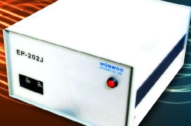
Developed by Wonwoo Systems Co., Ltd., EP-202J provides end-point detection (EPD) such as etching and deposition by monitoring and analyzing plasma gas spectroscopy in real time during production processes such as semiconductors, LCDs, and LEDs using Plasma.
