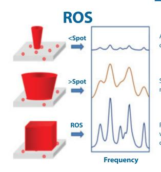
A tightly focused beam may give noisy signals or miss the Raman active target completely. This leads to false negatives from unidentified samples.
