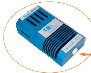
The LS-1-CAL-INT is calibrated specifically for use with the FOIS-1 Integrating Sphere. Notice the PTFE diffuser plug that's seated where an SMA 905 Connector is usually installed. This plug fits snugly into the sample port of the FOIS-1.
