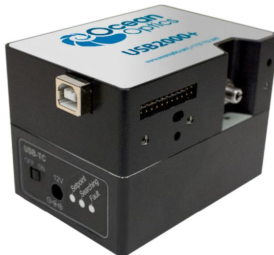
USB-TC Attached to a USB2000+ Spectrometer
