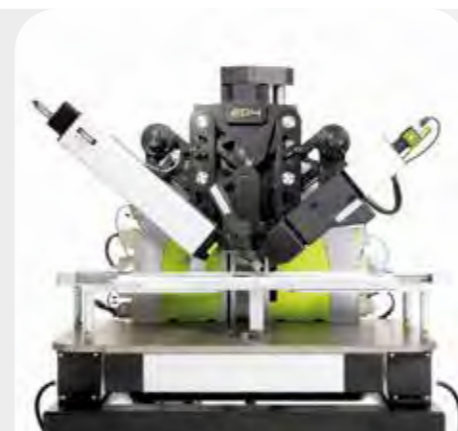
The nanofilm_ep4 with ultraobjective and KSV / NIMA trough
