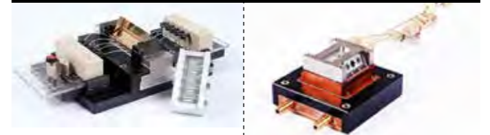
In situ SPR cell allowing kinetic SPR measurements
