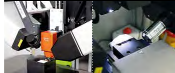
ep4 with adapted Nanosurf NaniteAFM
