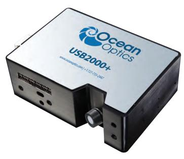
The USB2000+ Spectrometer is a clever combination of technologies: a powerful 2-MHz analog-to-digital (A/D) converter, programmable electronics, a 2048-element CCD-array detector and a high-speed USB 2.0 port.
